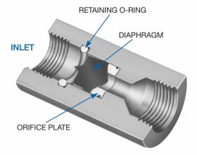
Single diaphragm design at left used for ¼ GPM through 8 GPM (.95 LPM - 30 LPM) constant flow rates. All higher flow rates use multidiaphragm design (consult factory for availability; minimums may apply).
