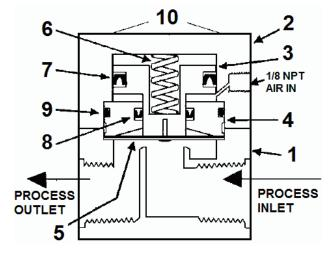
Shown as "NC" (Normally Closed). Spring will be under the piston and air will be directed over the piston for "NO" (Normally Open) valves.
