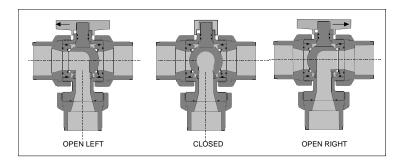
3-way ball valves with the three hole ball option are never closed. If the handle is in line with the piping, flow direction can be changed by turning the handle  $\frac{1}{4}$  turn clockwise or  $\frac{1}{2}$  turn counterclockwise. Turning  $\frac{1}{4}$  turn counterclockwise has no effect.
