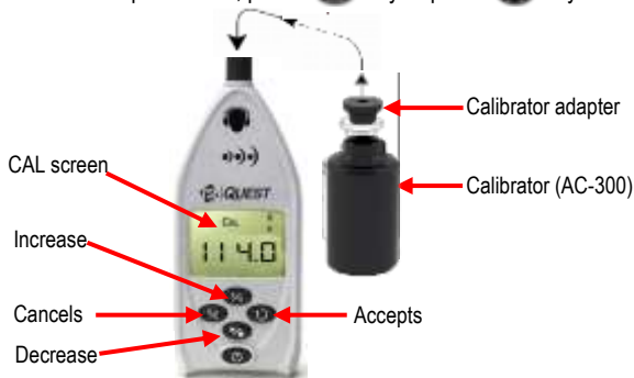
Figure 1-10: Calibrating the SD-200
