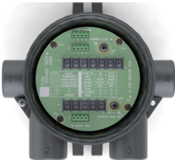
Figure 23 Junction Box Electrical Connections
