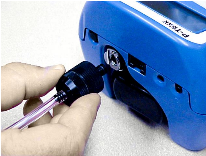
Figure 2-7: Insert Inlet Screen Assembly into Fitting
