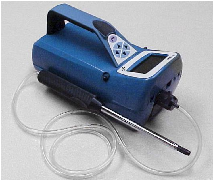
Figure 2-8: Slide Telescoping Probe onto Instrument Case
