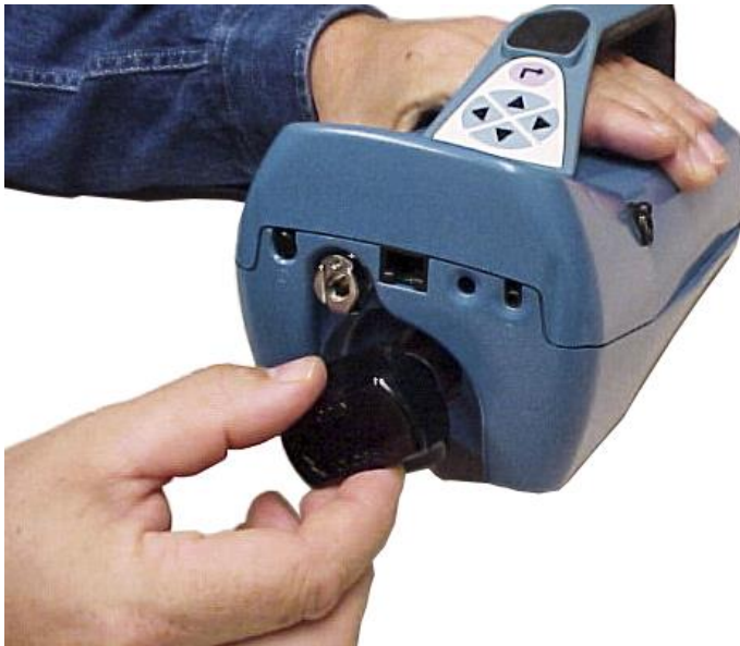
Figure 2-6: Insert Alcohol Cartridge into P-Trak Particle Counter
