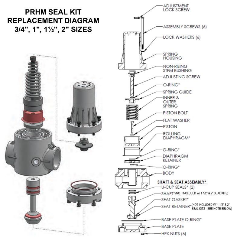
\* Asterisk indicates part included with Seal Kit. NOTE: The shaft and seat retainer are not included with the seal kit on the 1 1/2" and 2" size regulators. Unscrew the existing shaft and seat retainer and replace the old seat gasket with the new one included in the kit.
