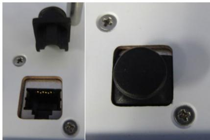
FIG 2 - Ethernet Plug Placement
