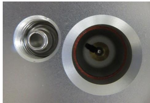
FIG 2 - Stage Tensioning Spring
