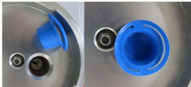
FIG 1 - Blower Inlet Plug Placement
