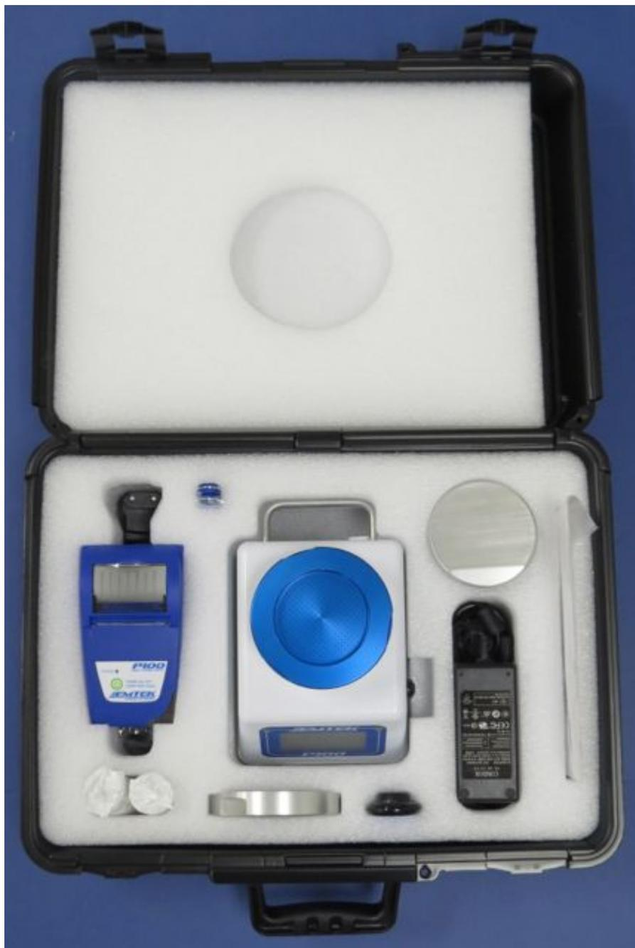
Fig. 1 - P100 Component Carrying Case
