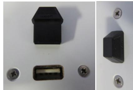
FIG 3- USB Plug Placement
