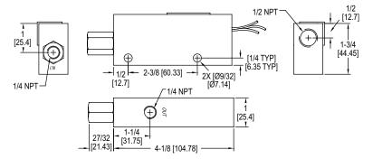
The Series P1 Brass Flow Switch utilizes a piston-type design for accurate detection of excessive or insufficient liquid flow rates. The switches have preset actuation points from 0.10 to 1.5 GPM for liquid flow.
