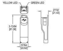
The Model MN-1 Mini-Node™ Communication Signal Converter is a economical device that converts half-duplex RS-485 serial communications signals into a signal that can be read by any computer with a USB port. The integral USB connector and RJ-45 connector reduces setup time by eliminating extra wiring. The Model MN-1 is powered via the USB connection which eliminates the need for an external power source. The compact size is great for field installation, control panels, and lab testing.
