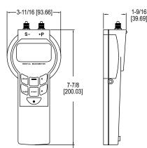
The Series HM35 Precision Digital Pressure Manometer is designed to reliably measure and log absolute pressure, differential pressure, or gage pressure with up to 0.05% accuracy. The data logging function can store up to 10,742 readings and transmit the readings to a PC through an IR serial port. The large display can graphically display trends in the data as well as peaks and valleys.
