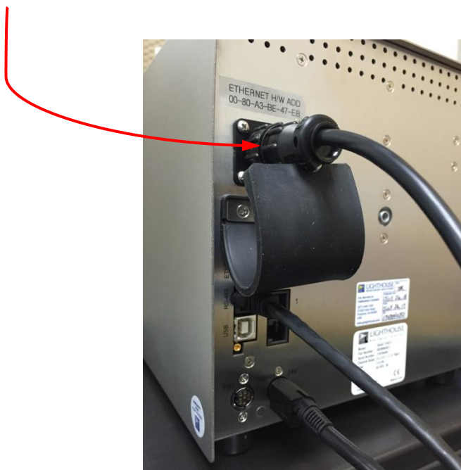
Figure 2-4 Connect Communication Cable to SOLAIR
