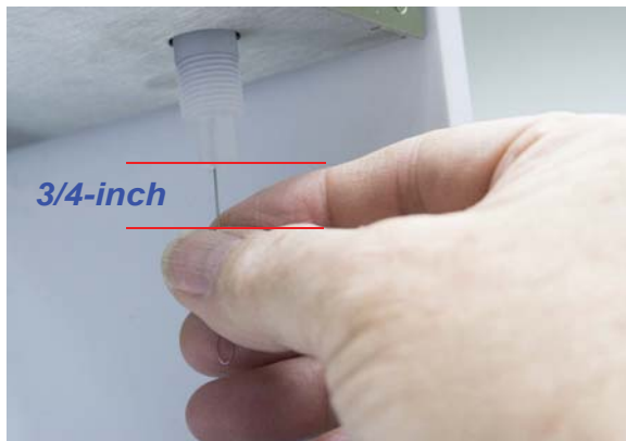
Figure A-1 Flow Cell Cleaning with 3/4-inch Limit
